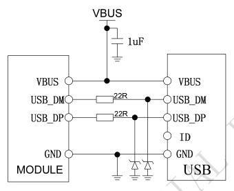
Figure 24: USB reference circuit
