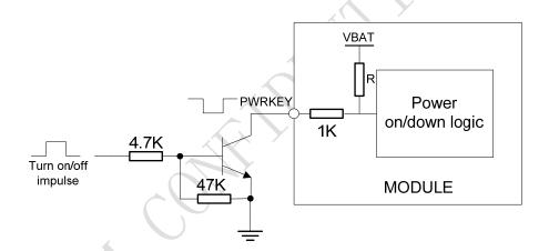
Figure 10: Powered on/down module using transistor
