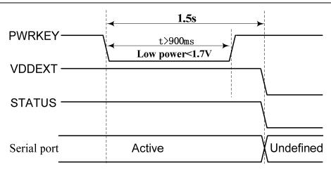
Figure 13: Timing of power down SIM800L by PWRKEY
