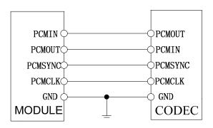
Figure 36: PCM reference circuit
