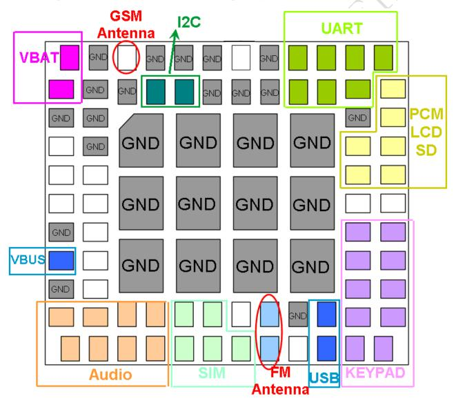
Figure 51: Pin assignment
