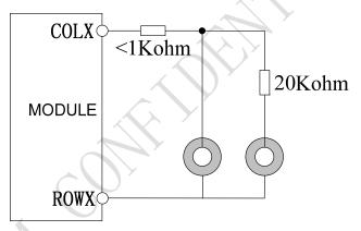
Figure 41: Keypad reference circuit
