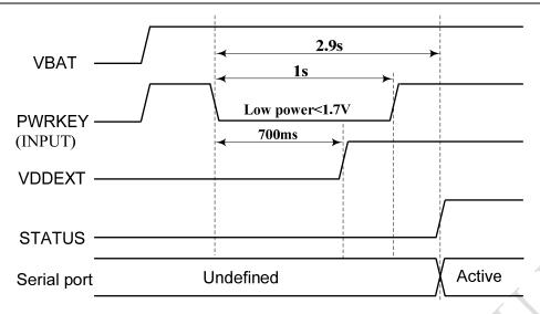
Figure 12: Timing of power on module
