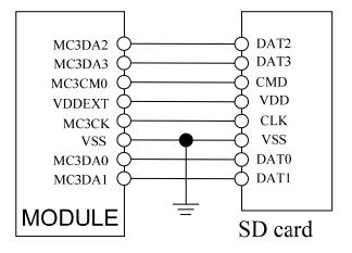
Figure 38: SD reference circuit
