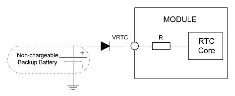
Figure 17: RTC supply from non-chargeable battery
