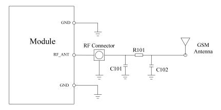
Figure 47: GSM antenna matching circuit
