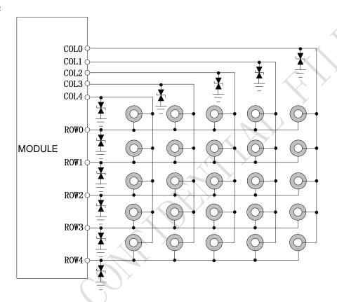
Figure 39: 25 keys reference circuit
