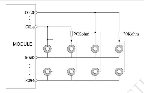
Figure 40: 50 keys reference circuit
