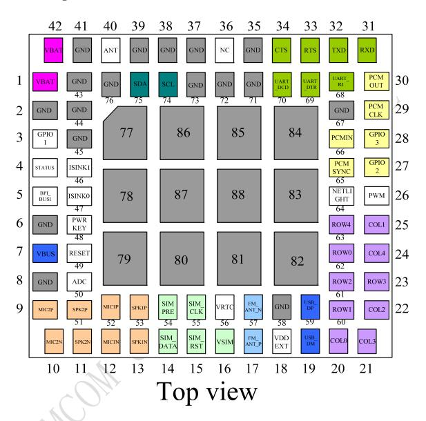
Figure 2: SIM800L pin out diagram (Top view)
