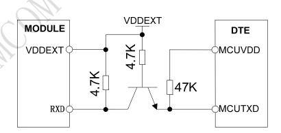
Figure 23: RX level matching circuit
