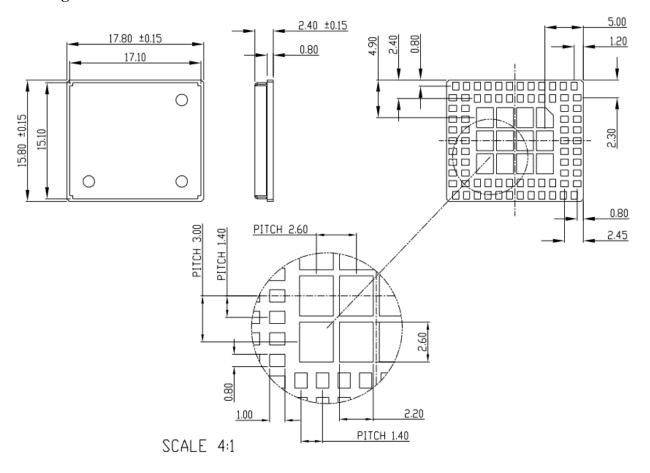
Figure 3: Dimensions of SIM800L (Unit: mm)
