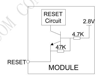
Figure 14: Reset circuit
