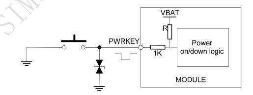
Figure 11: Powered on/down module using button
