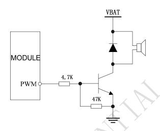
Figure 43: Reference circuit of PWM driver buzzer
