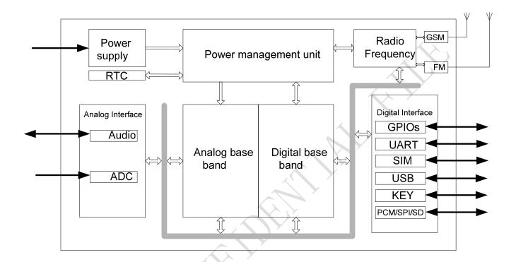
Figure 1: SIM800L functional diagram
