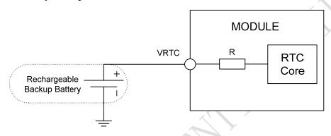
Figure 18: RTC supply from rechargeable battery
