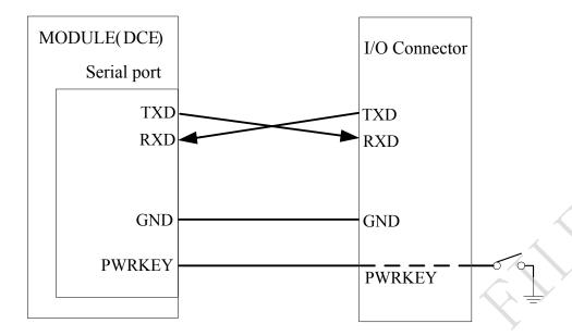
Figure 25: Connection for software upgrading and debugging
