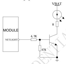
Figure 44: Reference circuit of NETLIGHT
