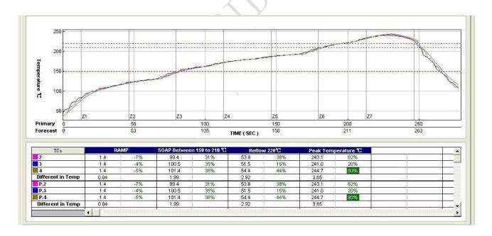
Figure 54: Typical solder reflow profile
