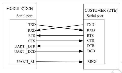
Figure 19: Connection of the serial interfaces
