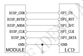
Figure 37: LCD reference circuit
