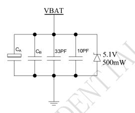
Figure 5: Reference circuit of the VBAT input
