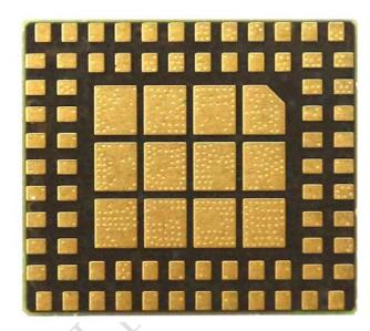
Figure 53: Top and bottom view of SIM800L
