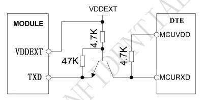
Figure 22: TX level matching circuit
