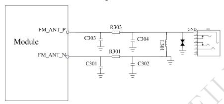
Figure 50: GND pin of the earphone use to be the FM antenna interface
