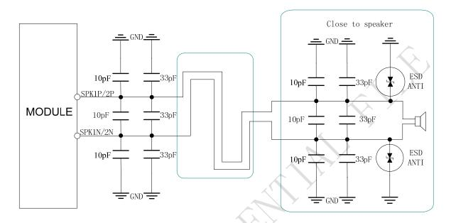
Figure 30: Speaker reference circuit
