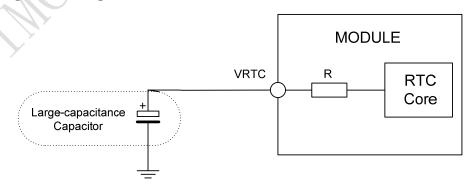
Figure 16: RTC supply from capacitor
