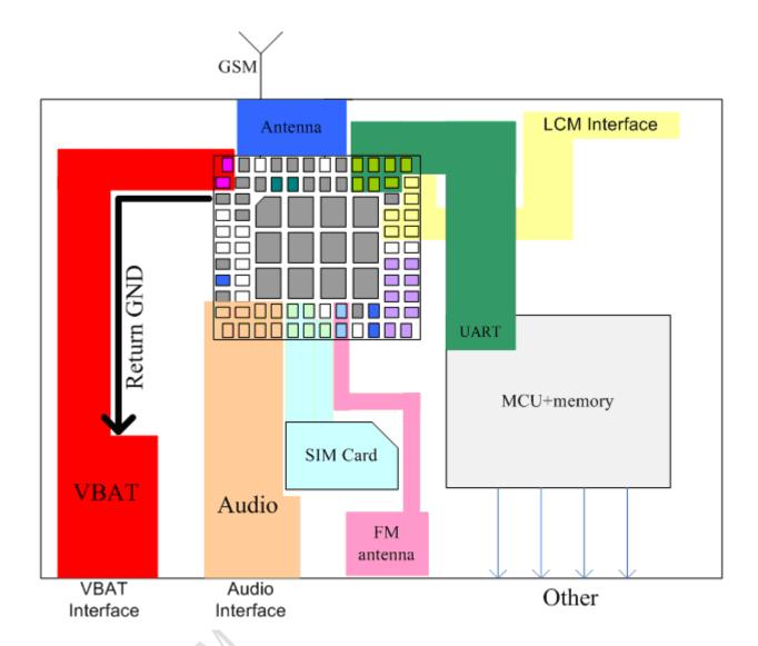
Figure 52: Recommended PCB layout
