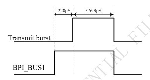
Figure 46: BPI\_BUS1 signal during transmit burst
