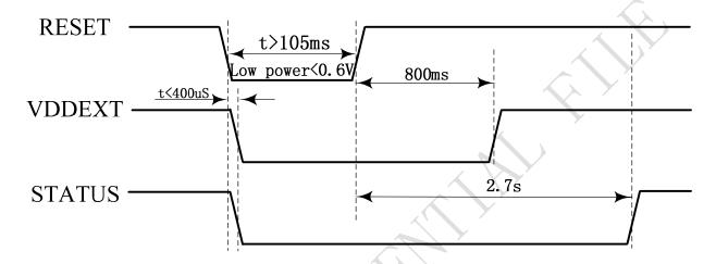
Figure 15: Reset timing sequence
