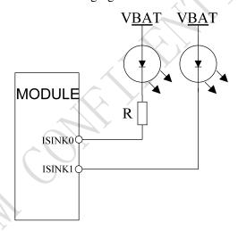
Figure 45: LED driver reference circuit
