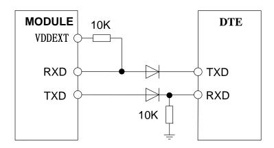
Figure 21: Diode isolation circuit
